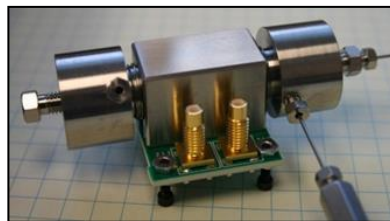
Figure 3: Sandia's miniPDID is about 1 x 1 x 2" in this embodiment, but can be made the size of a AA battery (Patent Pending).
